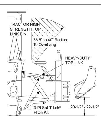
\* Operator's seat must be located in the lowest and most forward position to obtain 40" minimum radius.
